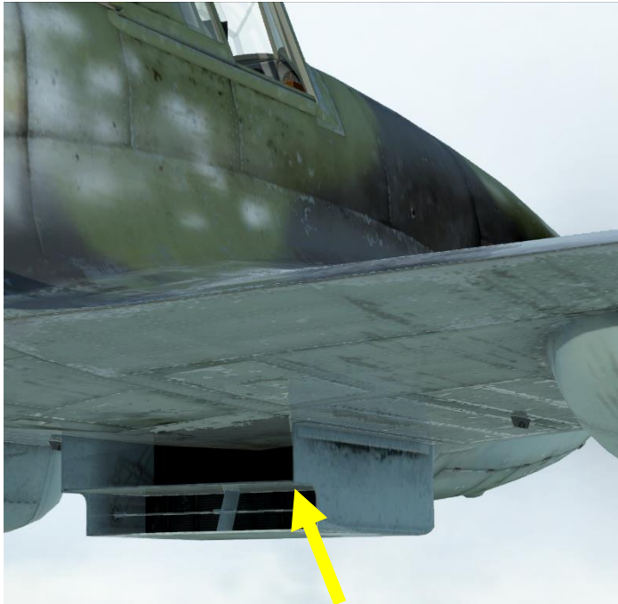
WATER RADIATOR OPEN
